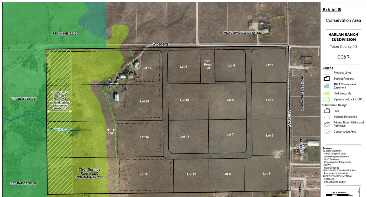
Figure 6. Restoration Plan – a 275 foot buffer will be passively restored to native emergent and scrub-shrub wetlands. The HOA will be responsible for monitoring the conservation area and documenting it.
