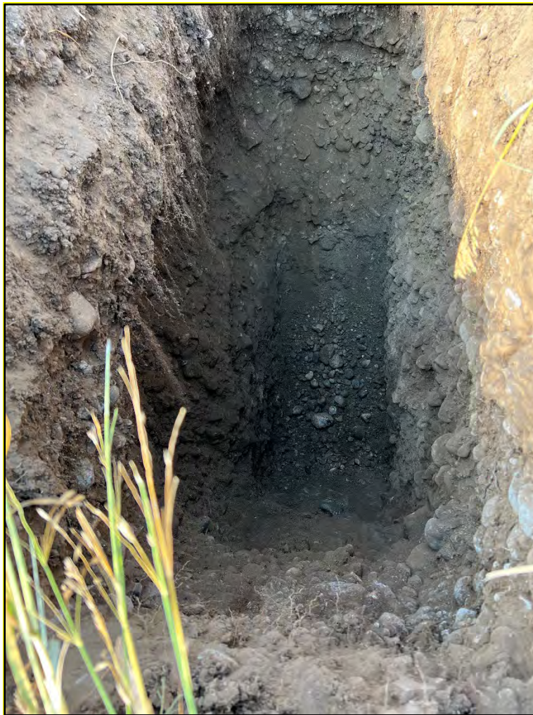
Figure 8. Test Pit Excavation
