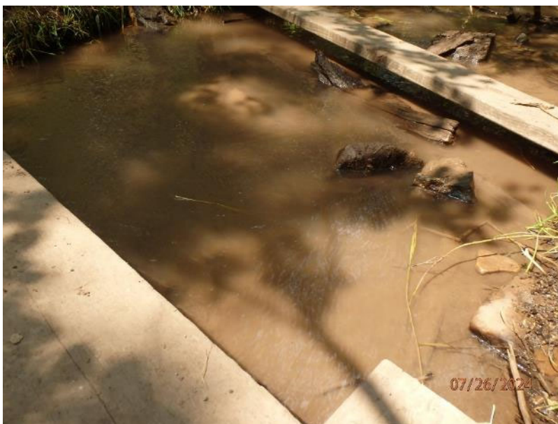
Figure 12. Photographic documentation of increased turbidity (of approximately 80 NTUs) on downstream property on July 26, 2024 (courtesy of DEQ).
